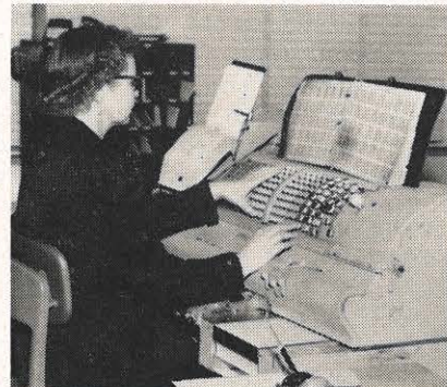
BILLING MACHINE OPERATION —The bill begins to take final form in the billing machine room. Mrs. Thelma Hiner copies the readings from the meter book and computes the charges by using a chart on the billing machine. The billing machine also prepares the ledger sheet, a control tape and a distribution tape. The machine is so designed that any error in subtraction will cause it to lock.
