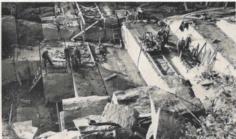
Typical of the many mineral deposits in the district, this soapstone quarry of the Alberne Stone Corporation helps enrich the area income. Workers manage the cutting machinery which saws the soft mineral into huge blocks at the quarry in the northern part of the district. (Photo by Fred Dudley.)
