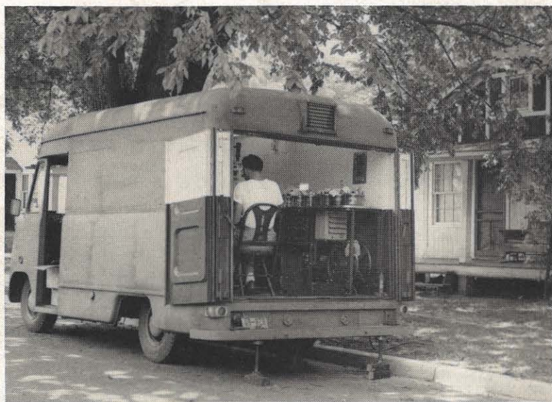
This photograph shows the new mobile meter testing laboratory which was recently put in operation in the Charleston district. The laboratory is shown in front of a customer's home ready to begin cleaning and testing meters in the neighborhood. Four jacks, two of which may be seen under the rear of the truck, are used to level and stabilize the laboratory.
