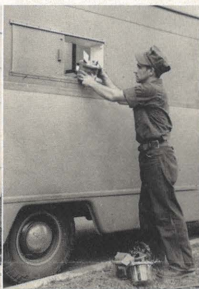
Bill hands the tagged meters through the window of the laboratory onto the repair table. The meters are carried to the mobile laboratory in special carriers which safely handle one to four meters.
