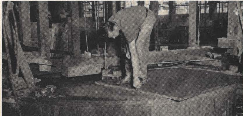
An Alberene employee checks the gauge of a slab being finished on the rotary rubbing bed. Abrasives and water cut the stone.
