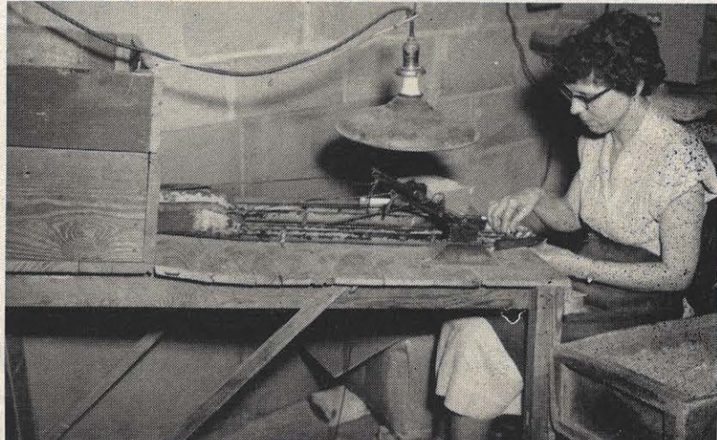
Bagging the marbles. An operator controls the flow of marbles going into the bag with the foot pedal. Filled bags are put in the box at right.
