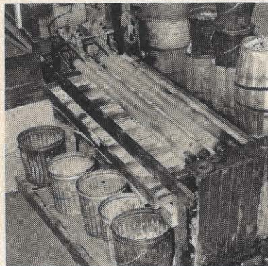
The sizing machine. Marbles in the box at top left roll over the revolving rollers which allow the small sizes to drop first. The marbles in the barrels and buckets in the background are yet to be sized.
