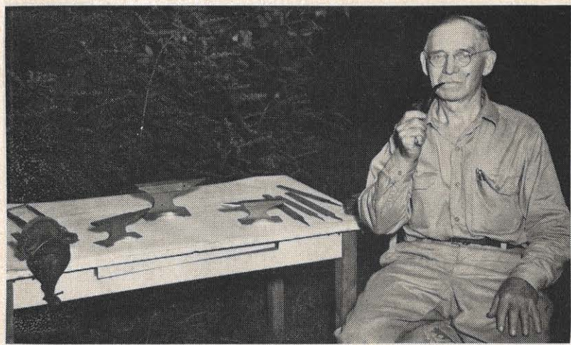
"Pop" displays some of the anvils he made at his workbench. He uses files, hacksaws and a grinding wheel to cut anvils from scrap ends of steel rails.
