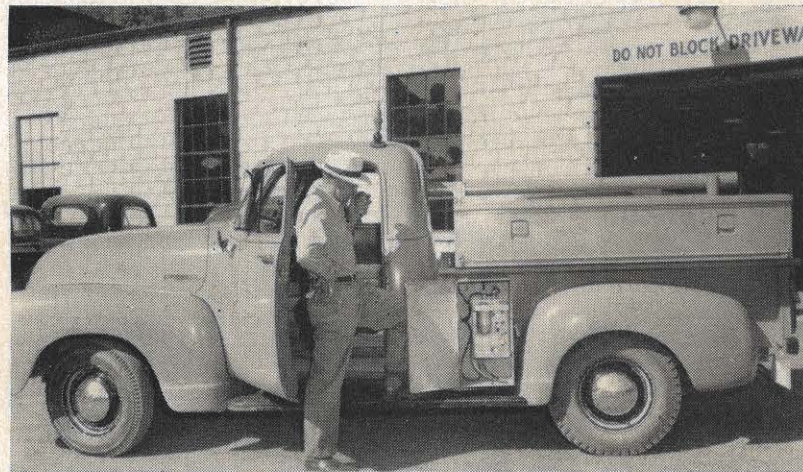
Two Abingdon district employees, R. P. Miller, transportation supervisor, and J. M. Orr of the substation department, solved their service trucks' space problems for the installation of two-way radio equipment. Two boxes are used on the sides of the truck. They are out of the way and do not alter the limited loading space. Above, A. C. Hutton, area serviceman, demonstrates the new installation on his truck.
