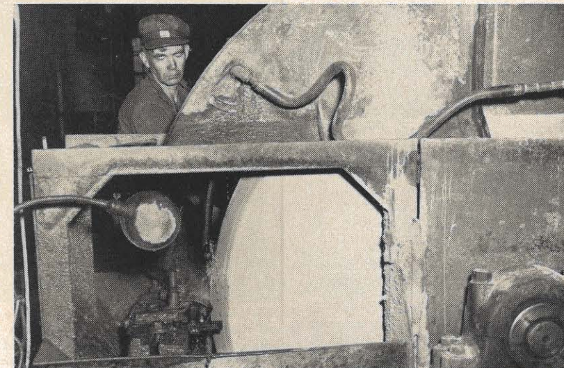
Using a grindstone. A worker at the Kelly Axe Works of Tru-Temper Corporation in Charleston sharpens a scythe blade on the whirling grindstone like those produced by the Constitution Stone Company.
