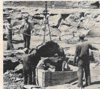
Hauling out an imperfect stone. As this part of the field was just beginning to be worked, the top layer is a softer grade of stone and sometimes shatters when blown loose with powder.
