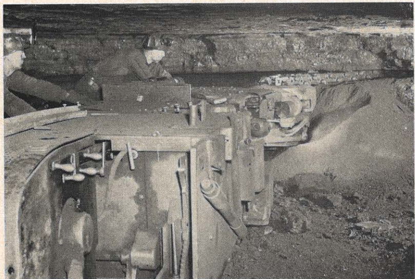
Miners are shown using an electrically-powered coal cutting machine. Such mechanization of mines has pushed production per man-day up more than 21 per cent in the last decade. The coal industry as a group is the largest industrial customer in the Southern Properties. They buy electricity to produce coal: we buy coal to produce electricity.
