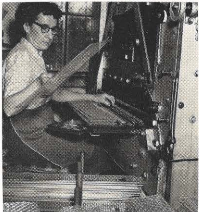
This Steelco employee operates the machine which presses angles and tabs into the wire mesh of the Steelco Gutter Screens.
