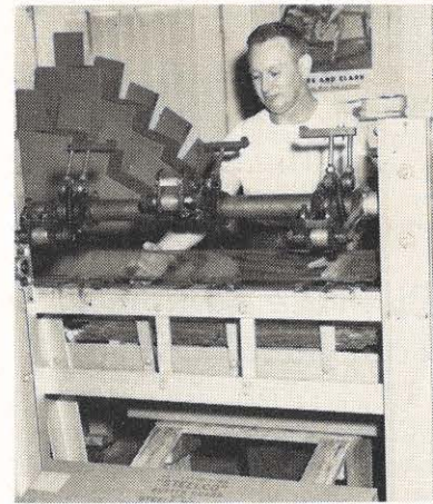
A Steelco worker completes the final operation in the fabrication of gutter screens. This machine punches and turns the tabs. All machines used in this operation were designed and built by the Steele Brothers.
