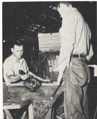
Final shaping of a Blenko vase is being done by one of the finishers. Initial shape was obtained by using an applewood mold.
