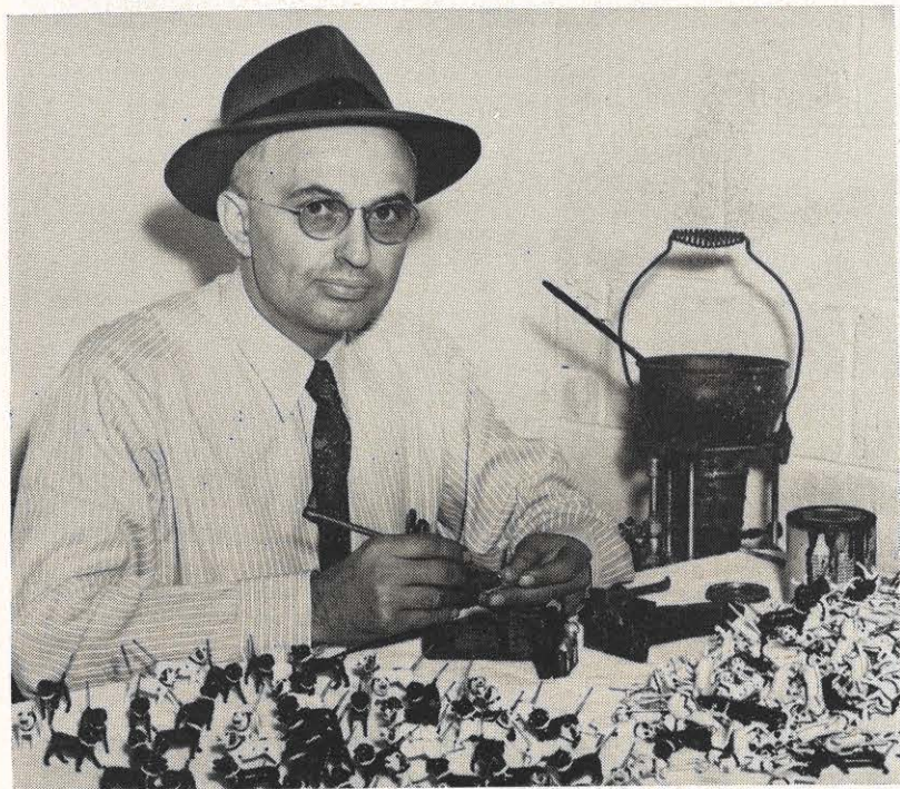
Putting the finishing touches on a pooch, J. W. Compton applies paint. A dog can be seen in the open mold. Several hundred finished products with spring tails that wag are scattered on the table in his basement.
