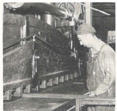
Cutting the heavy gauge steel used in building Oren fire engines from the chassis up is as easy as slicing cheese with this electric power shear.
