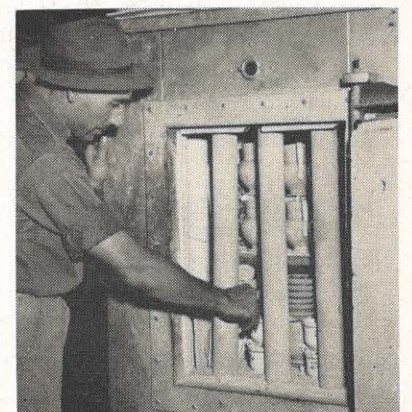
China is baked for 15 hours in this kiln at temperatures ranging from 1,500° to 2,700°, depending on the base of the paint. Stilts of fire clay are placed between each piece of china to keep them from touching.
