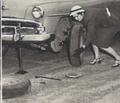
Sarah removes the flat tire from the hub, being careful not to jar the car. Notice how she has placed the hubcap holding the lug nuts and the jack handle out of the way so that neither will interfere with removing the tire. She rolls the flat tire to the rear of the vehicle and lays it on the ground.
