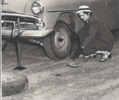
Before taking off the lugs and putting them in the hubcap, Sarah had placed the bumper jack in a firm position and jacked the car up, keeping to one side while pumping the jack with arm and shoulder in steady, even strokes. Sarah removes the lugs from the hub with the jack handle that doubles as a lug wrench.
