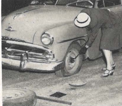
Before Sarah started loosening the lugs she got the spare tire, jack and screwdriver from the rear of the vehicle. She checked to see the handbrake was on and scotched the rear wheels with rocks. She removed the hubcap with the screwdriver. She is now just breaking the lugs loose, not unscrewing them or taking them off.
