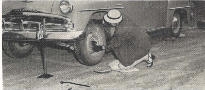
Having placed the inflated tire on the hub, she puts the lug screws in place, tightening them until all are firm against the base. She uses a newspaper to protect her knees and clothes while kneeling. She then clicks the jack gear into the down position and pumps the car down. She takes the jack to the rear and places it beside the flat tire to be sure not to drive off and leave it. She then finally tightens the lug nuts, puts on the hubcap and puts the flat tire and tools in the back. Finally, she takes out the rocks from under the wheels, gets in, takes a look up the road to see all is clear before she pulls out and gets going.
