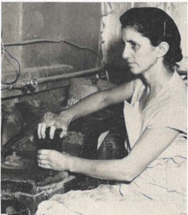
The bottle cut, Mrs. Edith Stephenson grinds off the sharp edges on an abrasive wheel. Then Ernest Stephenson puts on the final polish with an abrasive belt.
