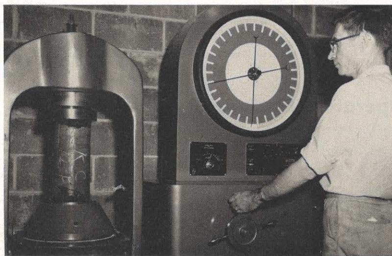
A cylinder is tested in a compression machine where it must withstand compression of at least 3,000 pounds per square inch before breaking. Ben Philson checks to see how the fly ash concrete holds up.
