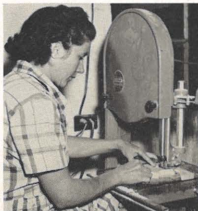
Bases are cut from cherry wood on a band saw by Mrs. Thelma Marrs.
