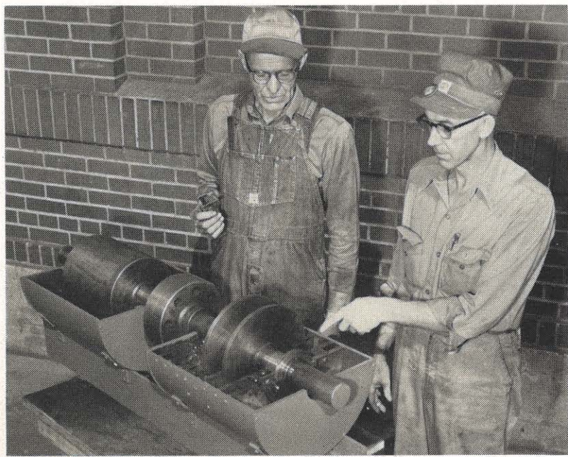
C. H. Feiszli points to a detail in the small model turbine which he and R. L. Boyd, left, built at Logan plant for training purposes. The model enables maintenance employees to study and get a better understanding of the correct procedures in the alignment of bearings, couplings and diaphragms. Feiszli is assistant supervisor of maintenance and Boyd is mechanical maintenance mechanic. With the model the main principles of alignment procedures can be studied at times other than when a turbine-generator unit is undergoing repairs.
