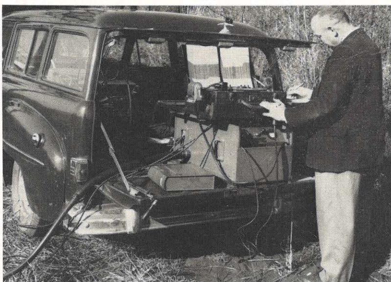
Checking the reports of a sick transformer is "Dr." John Campbell, test engineer. He serves as the diagnostician for the Beckley district, checking the "health" of each transformer at least once every three years.
