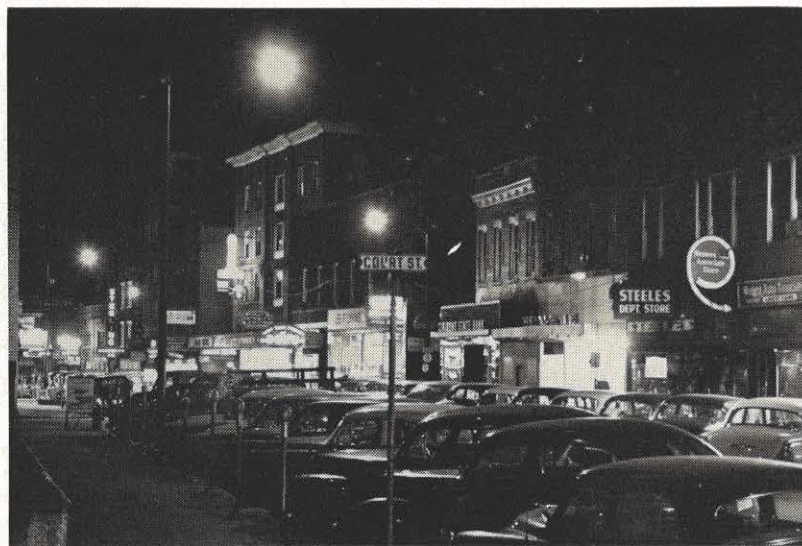
Downtown Hazard is lighted by photo-electric cells. Street lights in the picture were cut on automatically when the sun's light reached a low density point.
