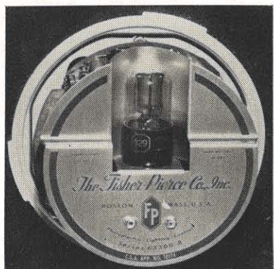
One of the many makes of photo-electric cells, this one has been stripped of its glass covering to show the electric eye, set in the center of the instrument. Resembling a meter, it uses a regular meter socket.
