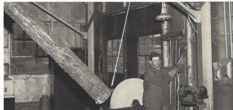
C. W. Hedrick raises the pole from the floor to its horizontal storage position with the help of a block and tackle.
