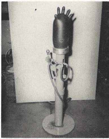
No, this isn't a "Shmoo." It's a rubber glove being inflated on the air testing device. Here any punctures or abrasions can be easily detected.
