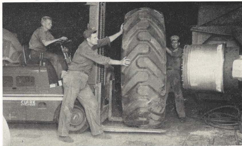
Changing a tire on a Euclid tractor at Sporn plant takes more than just a jack and lug wrench. Here, three men mount a new tire. James Russell operates the lift to move the huge tire into position while William Zerkle, on the left, and Ralph Rottgen help steady the tire being placed on the hub. Cost of the tire is over $2,000 and the recap price is over $1,000 each. Recapping is done in Alabama which is the nearest place to handle such a large tire. The tires are used on the Euclid coal moving equipment which weighs 31 tons and hauls 20 tons of coal per trip.
