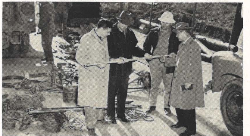
A hot stick gets a close inspection in Charleston by, from the left: John C. Frazier, safety supervisor; E. L. Smith, general foreman; Leroy Goode, line foreman; and E. H. Braid, distribution supervisor. The inspection committee and the line foreman are in the midst of a regular monthly check on tools and equipment at the North Charleston Service Building. On the third Thursday of each month service trucks are lined up and stripped of all equipment. And if a tool is found defective, it is either repaired or discarded. This shakedown method of eliminating unsafe working conditions, in this case defective equipment, is in addition to the on-the-job inspection of each piece of equipment before it is used.
