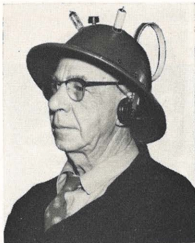
Is it a Space Cadet? Frank Buck? No. It's John Lindamood, veteran communications foreman of the Bluefield division, wearing a radio built into a pith helmet. John has been trying out the weird-looking gadget to locate radio interference. He says it works pretty well. The two "horns" are small radio tubes. The knob in front is a tuning dial and the loop on back is the antenna. Small batteries are worn in the pocket. Strange looking it may be, but John says "The Thing" is comfortable to wear.
