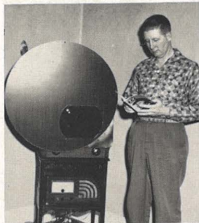
This unusual appearing apparatus enables J. P. Hughes to receive color television shows in color on his black and white set.
