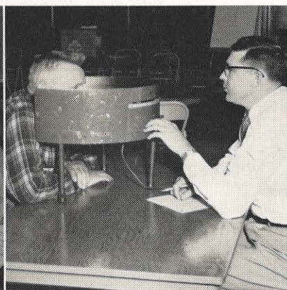
Looking much like a piece of face armor is this testing device being used on H. L. Bostic. John Frazier is conducting the test. The machine tells how close a moving object has to get alongside Mr. Bostic before he detects it. It is called, for that reason, a field of vision test. A poor score here indicates care is needed when changing lanes.
