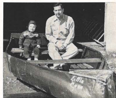
You might call it a hood boat. That's because Harold Coon, shown here with his son, Stephen Wayne, made "Little Coon" out of hoods from an old Cadillac and an old Oldsmobile. To these he added a 4 by 8 foot sheet of metal, two old bed rails, 30 feet of half-inch pipe, an acetylene torch and a lot of know-how. The Blue-field garage mechanic worked on the boat in his spare time this past winter "mostly because I wanted a boat to go fishing in." It will be launched this spring, and is built to take an outboard motor. The boat cost $12, a dollar for the pipe and $11 for the sheet of metal.
