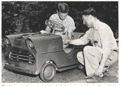
Checking over the sports car they built in seven months are Steve Hodges and Henry Altieri. The car with Plymouth lines is powered by a lawn mower motor in the rear and has a top speed of 12 miles per hour.
