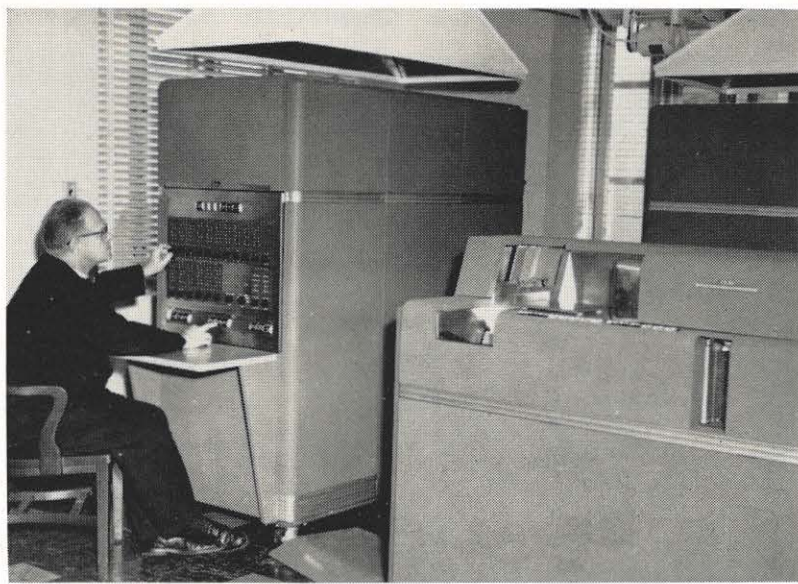
These three units make up the heart of the IBM system. Lawrence Ferguson, system billing supervisor, is operating the console unit of the 650 data-processing machine. The read-punch unit is at right with the power unit behind. The three units are interconnected by coaxial cables so they operate as one machine. Ducts above the units take off the heat generated.
