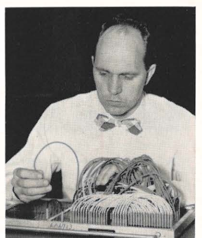
Earl Robertson is wiring a control panel for one of the IBM machines. Each control panel is wired to make the machine do a specific job. But by changing the panels, a machine will do many jobs.
