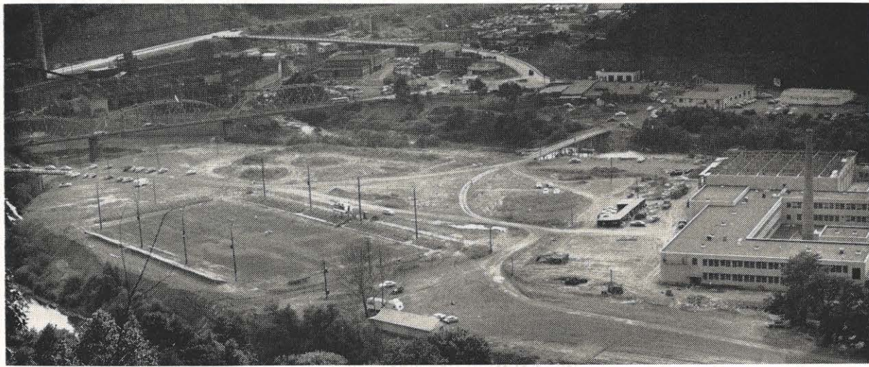
Underneath this school site is the lowly cinder, waste product of our plants. Cinders were pumped onto this island from Logan plant for four years, helping to build up and solidify the surface so that the high school, football field and other facilities could be built. Logan plant is at left and the Guyan River is visible around the island.
