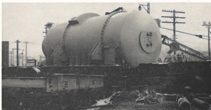
This piece of equipment weighs "only" 148 tons. It is a 50,000 kva, 11 kv synchronous condenser and will be installed at Turner transmission station in a $1-million expansion program. Turner, located at Institute in the Charleston district, is now receiving all materials necessary for the expansion. The condenser is shown on a siding, being prepared for transfer to a flat car for transporting to the foundation. Two low boys, with a total of 60 tires, and a bulldozer were required to move the condenser, largest in the Appalachian system and only the third one of its size ever built by Allis-Chalmers.
