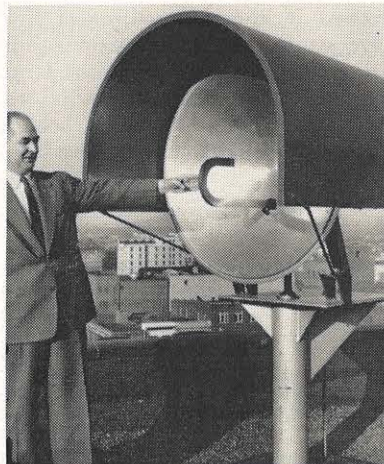
George M. Guill, system senior electronics engineer, touches the wave guide on the parabolic reflector atop the Roanoke office. This is one of the pieces of equipment being installed for the new microwave system between Roanoke and Charleston.
