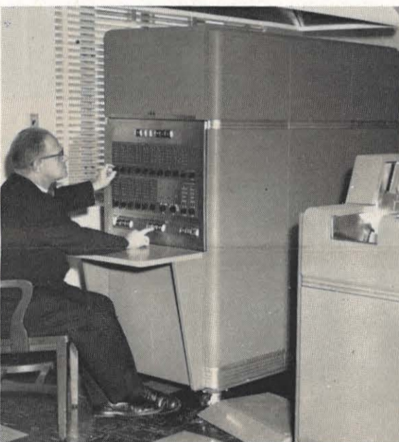
IBM electronic equipment was installed in Roanoke's general office building to take over billing for the three companies. Here Lawrence Ferguson, system billing supervisor, operates the console unit of the 650 data-processing machine, one of three main units. Coaxial cables connect this unit, the read-punch unit and the power unit so they operate as one.
