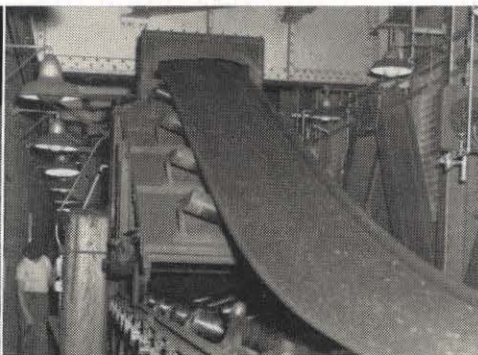
MIDDLE: Two coal handlers work at night to operate the conveyors and trippers which supply coal to the plant from the coal storage area. Here
