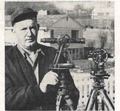
G. P. "Mac" Williams, Pulaski instrumentman, adjusts the 1890 transit his grandfather gave him. Although it is much larger than modern transit, rear, it has proven accurate.
