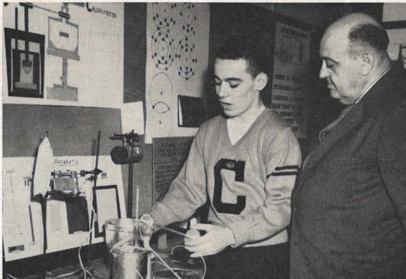
Virgil Brewer explains the calorimeter he built which recently won first prize at the Catlettsburg Science Fair Exhibit. The son of Virgil Brewer, Ashland district draftsman, young Brewer spent more than two weeks planning and about three days building this device which measures heat released by burning fuels. Here, he explains the apparatus to L. M. Kirk, a sponsor of the fair.
