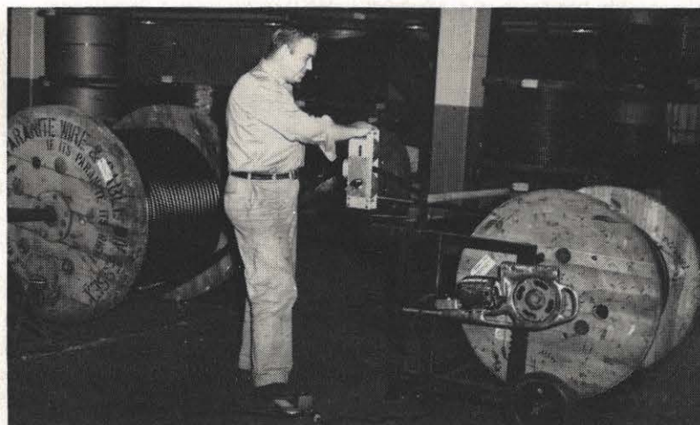
When cable is issued or returned to stock in our company storerooms it is necessary to measure the cable and reel it. Here, E. M. Payne, Roanoke head material clerk, demonstrates new wire handling equipment to do these jobs. One man, using this equipment, can do in 10 or 15 minutes what previously required three or four men forty minutes to do. The equipment is power driven, and handles control, copper and aluminum cable.
