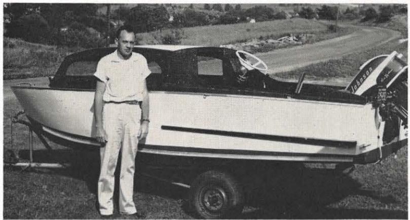
W. L. Smythers, Abingdon district engineering aide, stands beside the 15-foot outboard cruiser he built and named "The Disagreeable." Mr. Smythers started construction of the boat last November and completed it in April. The framing is white oak, and the sides and bottom are fibreglas-covered marine plywood. The cabin has 46-inch head room, a 72-inch beam and sleeps two adults. Accessories include remote control steering and throttle, rails and running lights. It is pushed by a 35 horsepower motor.
