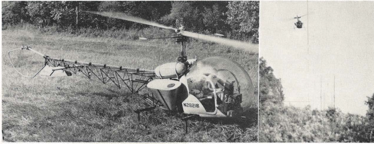
LEFT: Preparing for take-off with loaded spray tanks is this whirlybird, used to spray right-of-way on a Pikeville district line. A funnel-shaped spray tank can be seen in the middle of the copter. RIGHT: Spraying along the David-Falcon 46,000 volt line, this helicopter whirls along only six or eight feet above the circuit.
