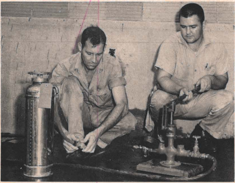
A hydrostatic test pump to check the reliability of foam and cartridge-operated water extinguishers has been put into service at Kanawha River plant. Showing how the tester is connected to an extinguisher are F. W. Holdren, left, and C. W. Crawford. The National Board of Fire Underwriters Standard provides for a pressure checking of extinguishers periodically.
