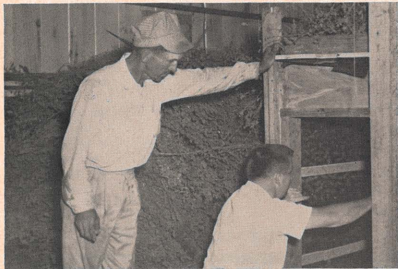
Larry L. Bucklen, right, Pulaski agricultural engineer, checks the air duct which supplies air to dry catnip. The catnip itself is behind Charlie Thomas, a tenant on the George W. Greer catnip farm.
