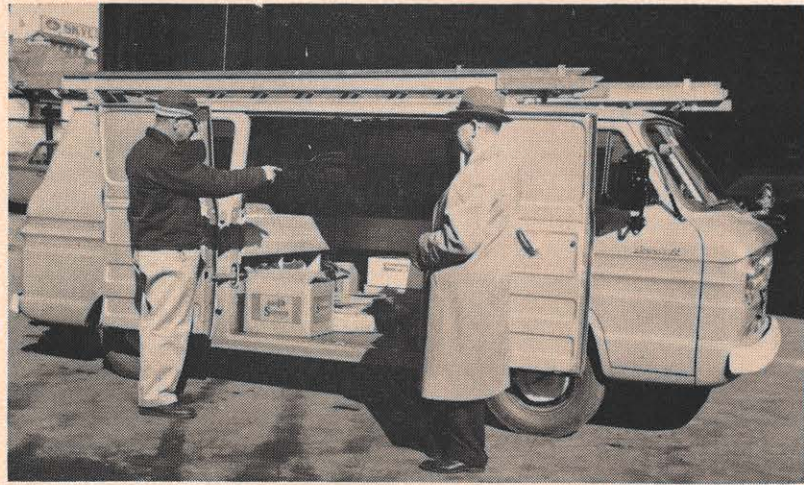
This new type of meter service truck is now in service in the Roanoke district. A panel truck based on the compact principle, it offers low initial cost and operating economies as well as efficient loading and storage. Special bins were installed inside the truck for miscellaneous parts, and a double ladder rack on top for two extension ladders. Both the rear and side doors of the unit open back against the body, permitting the operator easy access to the contents. Completely enclosed, the truck gives protection to all materials. Here, P. A. Grisso, meter serviceman, left, and E. W. Holland, meter service foreman, look the truck over.
