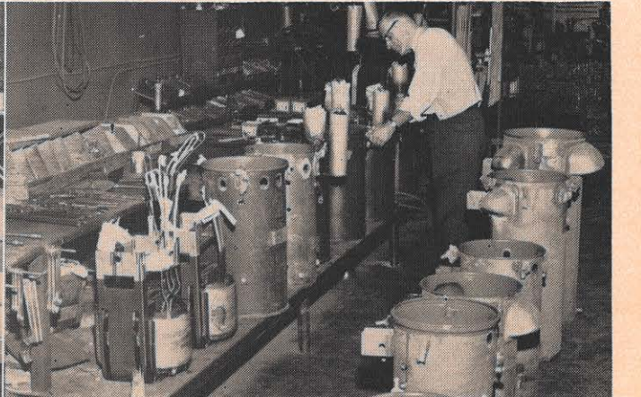
In this Westinghouse repair shop, transformers are rebuilt with new coils, cores, bushings and gaskets and get coatings of paint inside and out. Shown inspecting the "old into the new" is Mr. Whitekettle, shop foreman.
