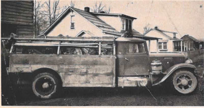
Bluefield district's first line construction and maintenance body truck—above—was designed by W. P. Carter, now system transmission line superintendent, in 1928. Before that the trucks used were simply stake body trucks. Oscar Adams, Princeton area supervisor, ran across this photo in some old records recently. Strangely enough, the design of compartments and doors has changed little since those days, and even the water keg next to the hood—a "wagon train" touch—has its counterpart today in a vacuum jug. Laurence B. Riggs, present line inspector in the district, drove the truck for many years.
