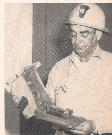
S. R. McClure, Welch line foreman, holds the 1926 version of a line fuse cutout box discovered in operation in Davy.
