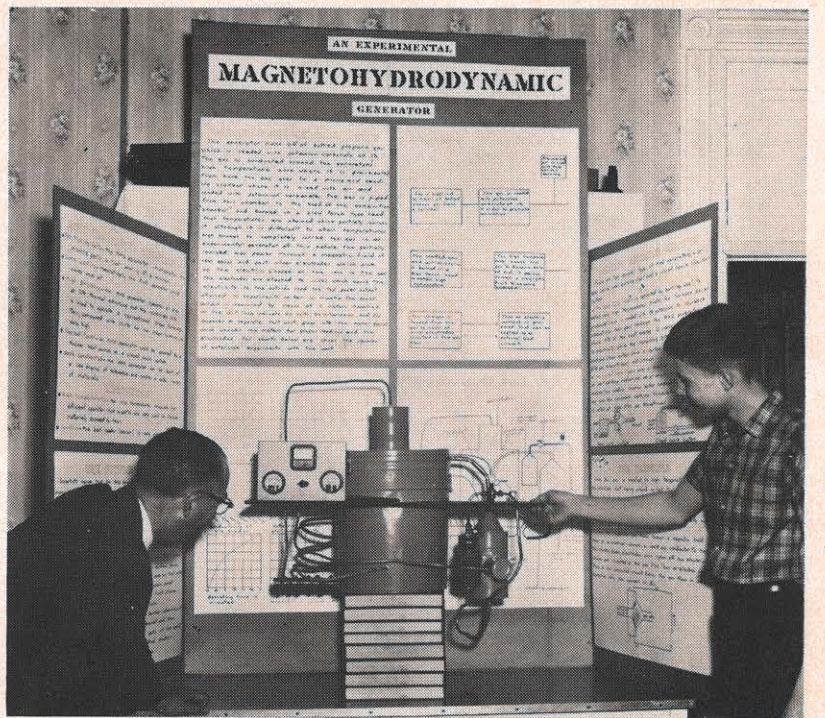
Aubrey Strode shows G. M. Guill, Jr., assistant system supervising electronic engineer, how his MHD generator works. In this picture the generator has been placed on a stack of books and its housing removed in order to show its construction.
