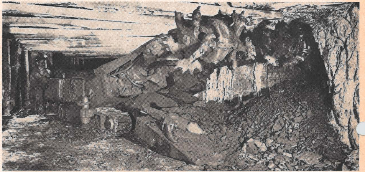
A continuous miner works at a seam of coal in a contributor to the economy of the Bluefield district's mine in the Bluefield area. Coal remains a chief general area.
