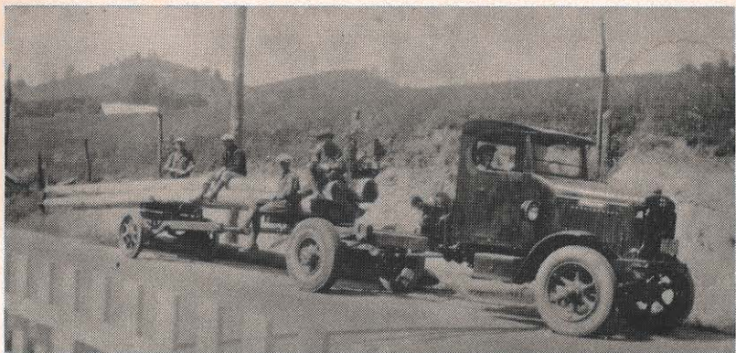
Thirty-six years ago, a Clinch Valley district all-purpose line truck looked like this. C. M. "Tip" Fletcher (in white cap), Bluefield line supervisor, who supplied the picture, reports that after poles were delivered, a truck bed, hanging from an apple tree, was lashed onto the trailer, and loaded with men and materials for the next job. James Butler, retired, is on the end of the poles with Mr. Fletcher, and E. B. "Red" Brewer, lineman, is looking out of the cab window.
