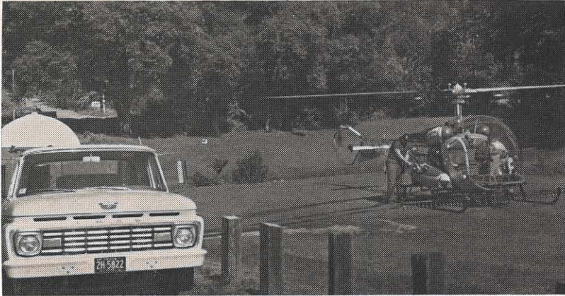
Aerial spraying of transmission lines in Hazard has been completed, thanks to swift operations like the one shown above. The entire refueling operation, in which the helicopter takes on new loads of chemicals, gas, and oil, takes less than a minute.
