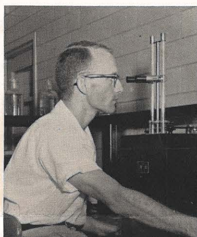
Mr. England peers through a magnifying glass to read thermometer inside the calorimeter, a precise instrument used to measure the heat content of coal.
