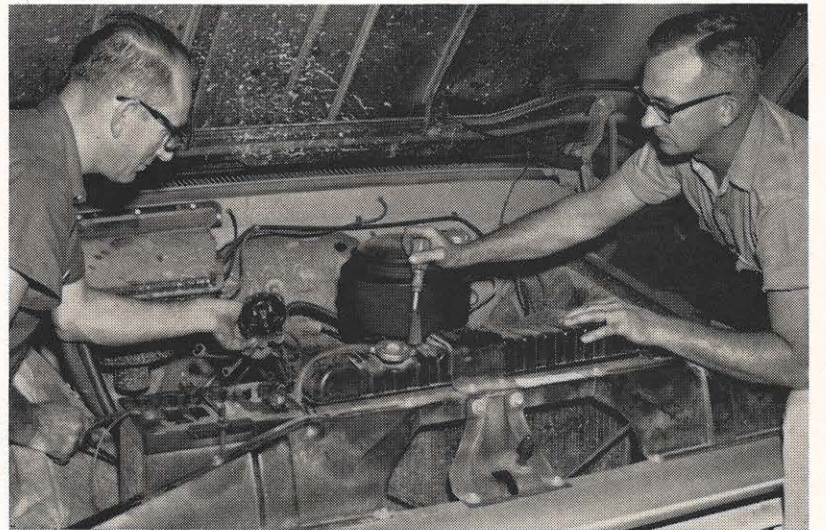
C. N. Chapman and T. R. Templeton inspect the distributor cap on a truck in the Huntington division garage. They help in the care and feeding of 75 trucks and cars.
