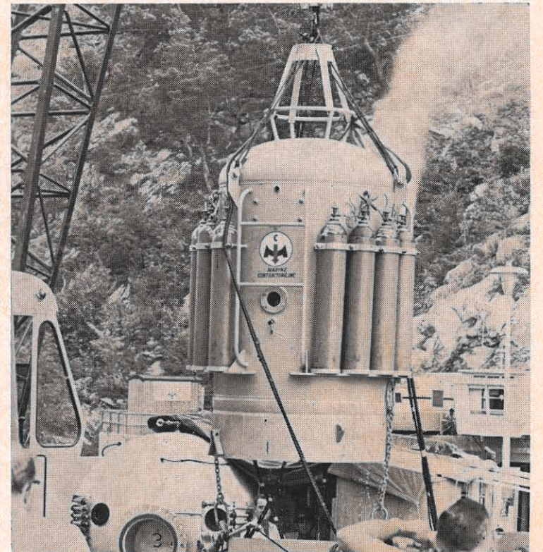
ing live in this chamber under pressure. A hatch—the circle with "3" painted on it—connects the capsule and the chamber to per-
