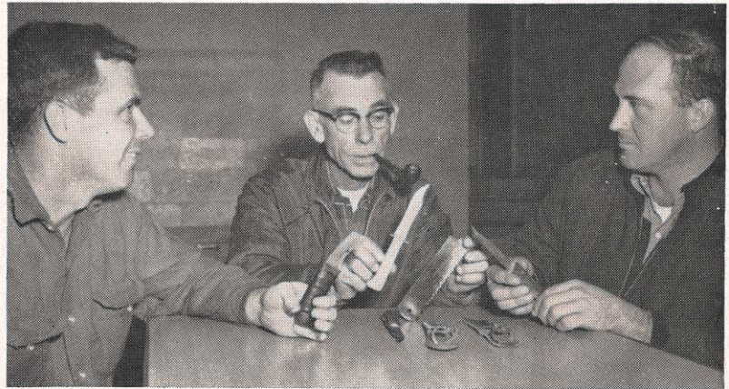
T. K. Rhodes, center, Charleston truck driver-groundman, shows off to Red Holmes and Tommy Young some of the knives he has made and used over the years. He makes the knives out of old metal-cutting saw blades; and they can be used for cutting wire, and never need sharpening. About 25 linemen in the division now use the knives. Red Holmes, left, is holding one.
