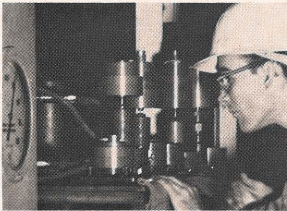
John Hunt measures turbine pressure with dead weight gauges during a heat rate test.
