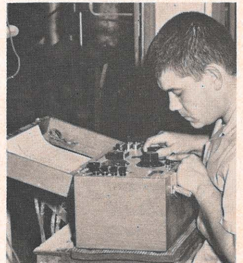
Harold Cook uses a potentiometer to measure temperature during a heat rate test.
