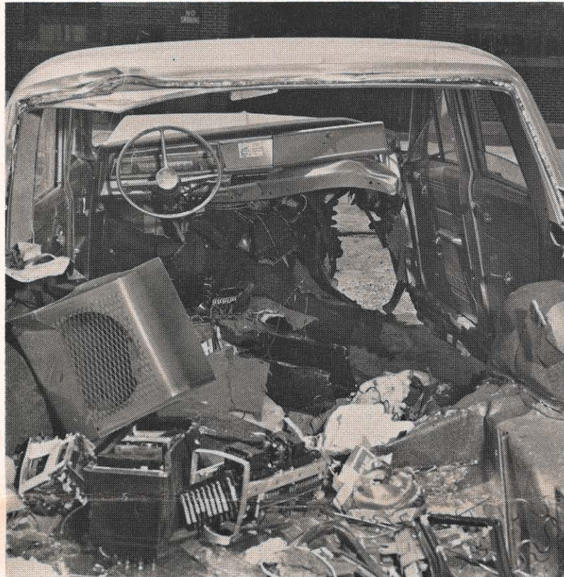
Interior ripped clean by guardrail
