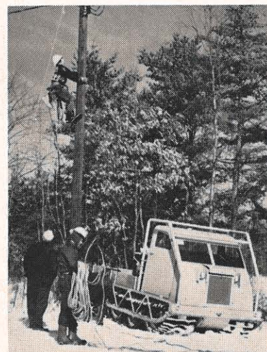
Roanoke division Bombardier Carrier was put into use to reach areas where rugged terrain and snow prevented other methods of transportation.
