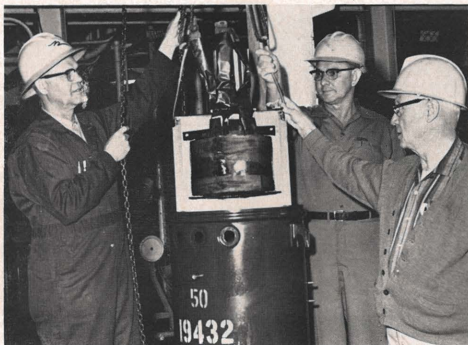
A new 50-kva transformer failed in service. H. H. Perdue (from left) Claude Thompson and Frank Lake are charged with the responsibility of determining "why."
