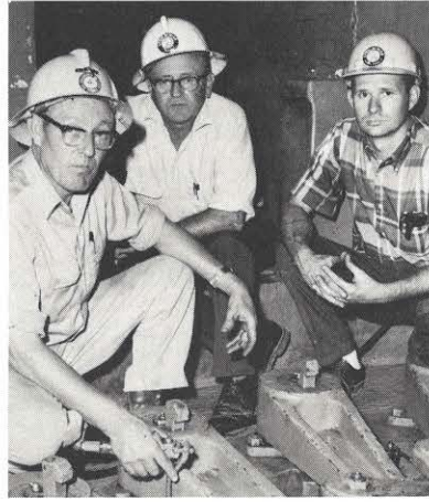
Dallas Spraker (left), Buford Sharp and Paul Askew take a look at grease fittings which are now readily accessible to a maintenance man with a grease gun.
