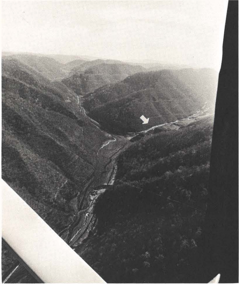
The slag dam which broke, sending millions of tons of water rushing through the valley, is indicated by the arrow. This aerial shows approximately the first four miles below the dam, which was completely devastated. Photo courtesy Huntington Publishing Company.
