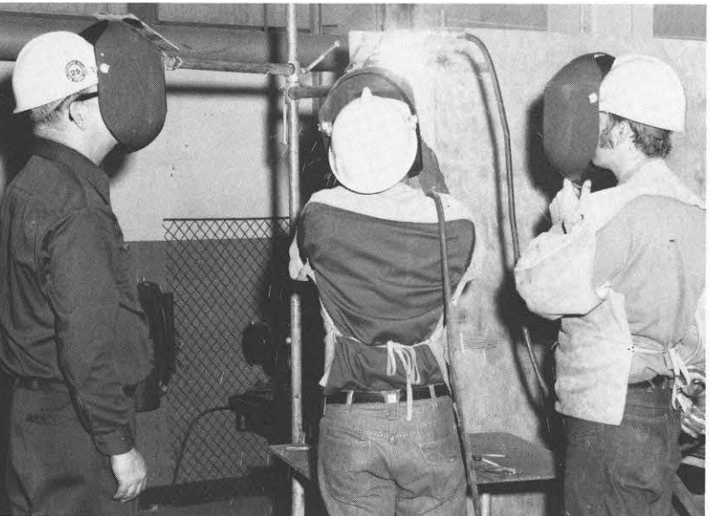
To fill the company's need for certified welders, Appalachian Power's General Office Training Section is using a programmed learning course developed by Westinghouse Learning Corporation. Entitled "Basic Arc Welding", the course includes 12 tapes which show on an audio-visual set the step-by-step method of welding in four ways: flat welds, vertical welds, horizontal welds, and overhead welds. After the tapes are shown, actual welding is
