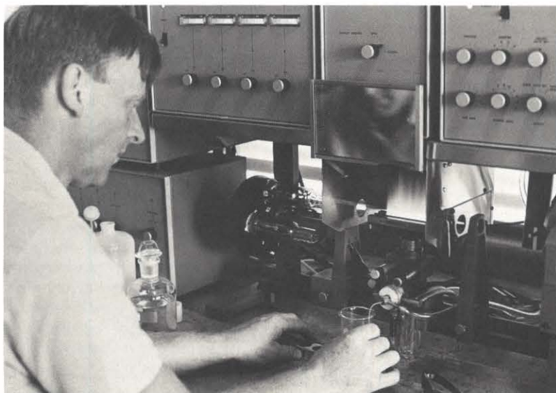
Bill Rowley isolates trace metals on the atomic absorption spectrophotometer.
