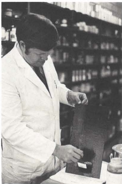
Bill Harbour brushes on a rust converter to study its performance.
