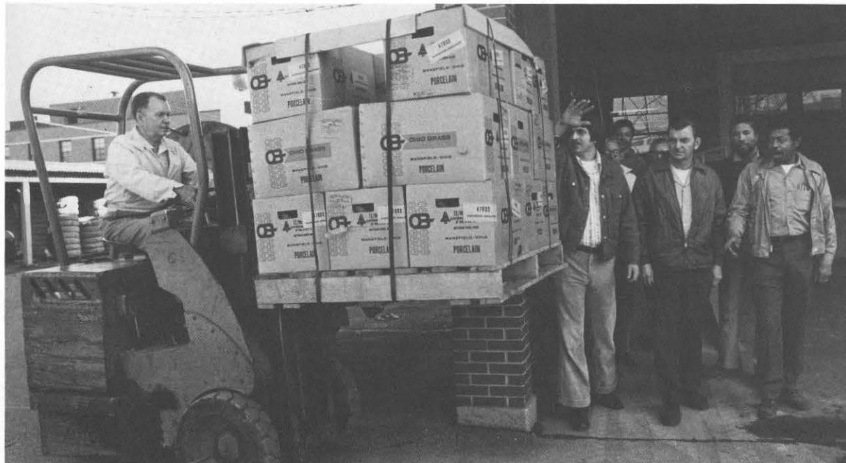
Operator Vick Altizer is carrying a load so high that he cannot see the employees about to walk into his path.
