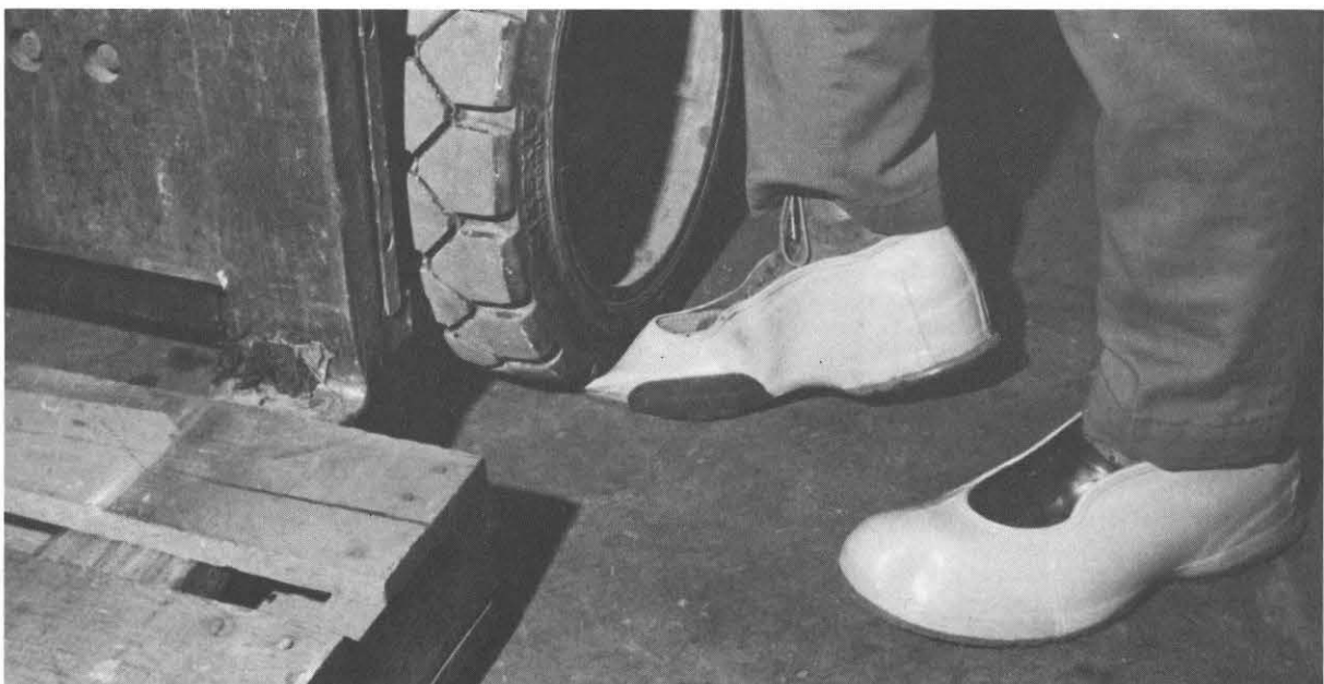
Employees working around a fork lift should be especially careful not to get caught in a situation like this one.
