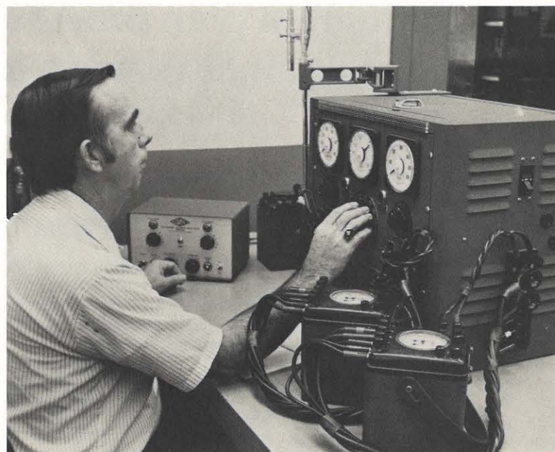
Wayne E. Webb, T&D meterman A in the General Office Meter Section, Roanoke, makes a comparison test of a division meter kwh standard against the General Office reference standard.
