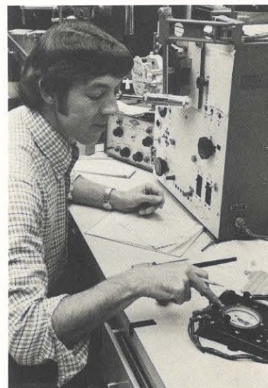
Bill H. Eller, Jr., Roanoke Division meterman A, tests one of the 1600 sample meters selected by the computer for checking in Roanoke Division last month.
